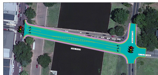
Replace Cane River Bridge on Skewed Alignment Without Temporary Bridge
