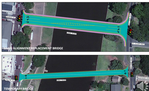
Replace Cane River Bridge on Same Alignment with Temporary Bridge at Touline Street
